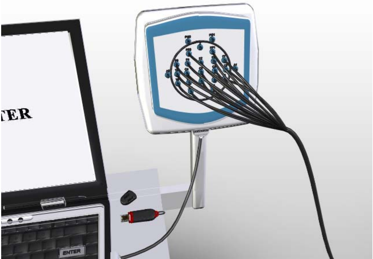
Figure 6. Electrodes connection to the amplifier
