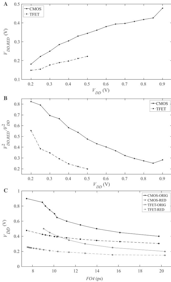
**FIGURE 2** Impact of concurrency on  $V_{DD}$  and  $PR$  for FinFET and TFET technologies. A,  $V_{DD}$  reduction, B,  $PR$  versus  $V_{DD}$ , and C,  $V_{DD}$  versus  $FO4$  delay. TFET, tunnel field-effect transistor
