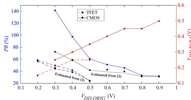
**FIGURE 3**  $PR$  (%) and  $V_{DD,PARA}$  versus  $V_{DD,ORIG}$ , including the  $PR$  (%) versus  $V_{DD,ORIG}$  estimation from expression 2. TFET, tunnel field-effect transistor [Colour figure can be viewed at [wileyonlinelibrary.com](http://wileyonlinelibrary.com)]
