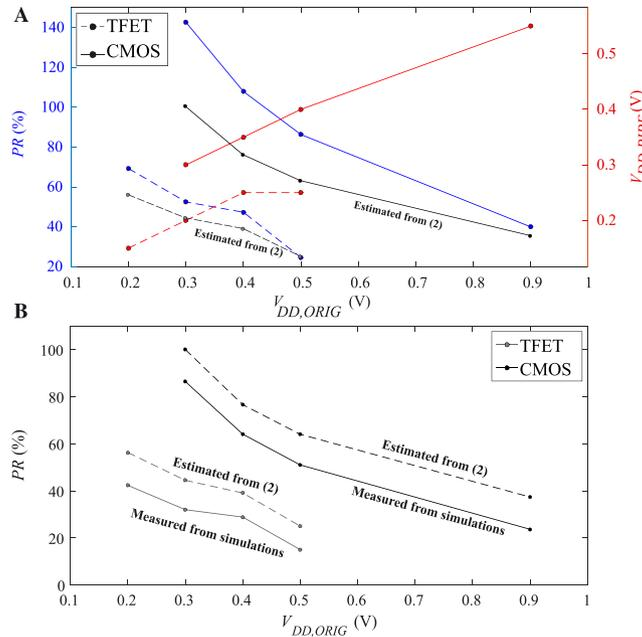
**FIGURE 4** A, PR (%) versus  $V_{DD,ORIG}$  and  $V_{DD,PIPE}$  versus  $V_{DD,ORIG}$  plots. B, PR (%) versus  $V_{DD,ORIG}$  without considering the impact of pipeline registers. TFET, tunnel field-effect transistor [Colour figure can be viewed at [wileyonlinelibrary.com](http://wileyonlinelibrary.com)]
