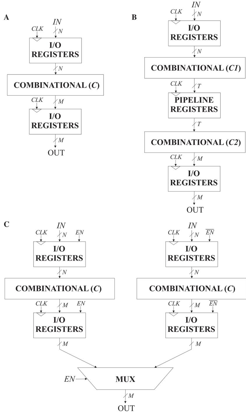
**FIGURE 1** Block diagrams illustrating A, original implementation, B, pipelining, and C, parallelism
