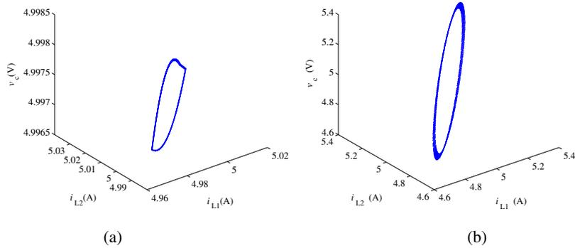
Fig. 2. 3-dimensional trajectories. (a) Stable period-1 trajectory for  $K_1 = K_2 = 1.9$ ,  $\tau_{F1} = \tau_{F2} = 0.3/\omega_0$ ,  $K_i = 1$ ; (b) quasi-periodic trajectory after the slow-scale bifurcation for  $K_1 = K_2 = 2$ ,  $\tau_{F1} = \tau_{F2} = 0.3/\omega_0$ ,  $K_i = 1$ .
