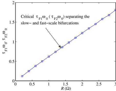
Fig. 5. Critical  $\tau_{F1}\omega_0$  ( $\tau_{F2}\omega_0$ ) separating the slow- and fast-scale bifurcations for different output power levels with  $K_i = 1$ . For  $\tau_{F1}\omega_0$  ( $\tau_{F2}\omega_0$ ) below the critical value, slow-scale bifurcation occurs as  $K_1$  ( $K_2$ ) is increased. Fast-scale bifurcation occurs otherwise.
