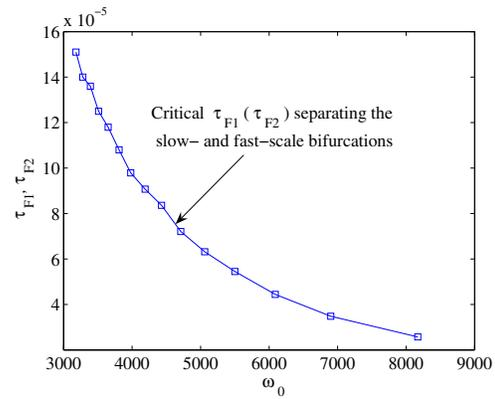
Fig. 6. Critical  $\tau_{F1}$  ( $\tau_{F2}$ ) separating the slow- and fast-scale bifurcations for different  $\omega_0$  with  $K_i = 1$ . For  $\tau_{F1}$  ( $\tau_{F2}$ ) below the critical value, slow-scale bifurcation occurs as  $K_1$  ( $K_2$ ) is increased. Fast-scale bifurcation occurs otherwise.
