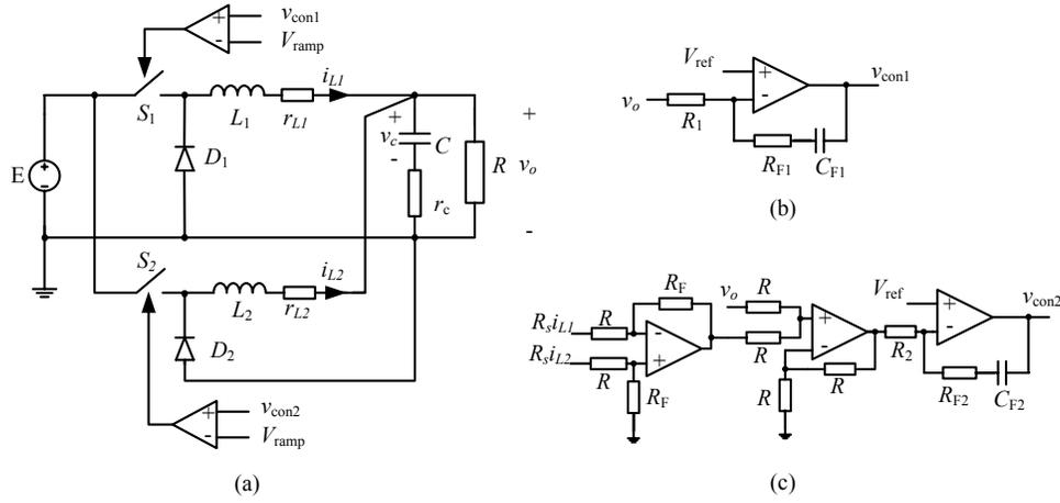
Fig. 1. Parallel connected buck converters under master-slave current sharing and PI control. (a) Converter stage; (b) controller for the master; (c) controller for the slave.
