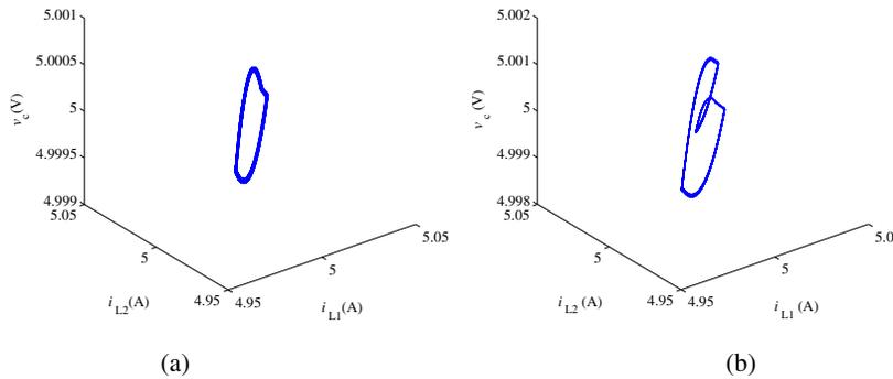
Fig. 3. 3-dimensional trajectories. (a) Stable period-one trajectory for  $K_1 = K_2 = 560.5$ ,  $\tau_{F1} = \tau_{F2} = 1/\omega_0$ ,  $K_i = 1$ ; (b) period-2 trajectory after the fast-scale bifurcation for  $K_1 = K_2 = 561$ ,  $\tau_{F1} = \tau_{F2} = 1/\omega_0$ ,  $K_i = 1$ .
