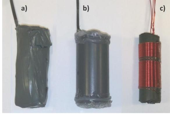
Fig. 3. Sensors with and without isolating cover
