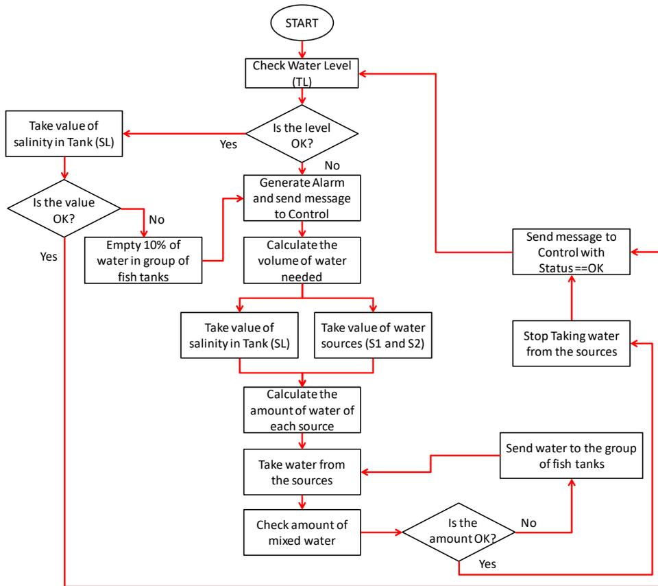
Fig. 12. Flow diagram to control the system
