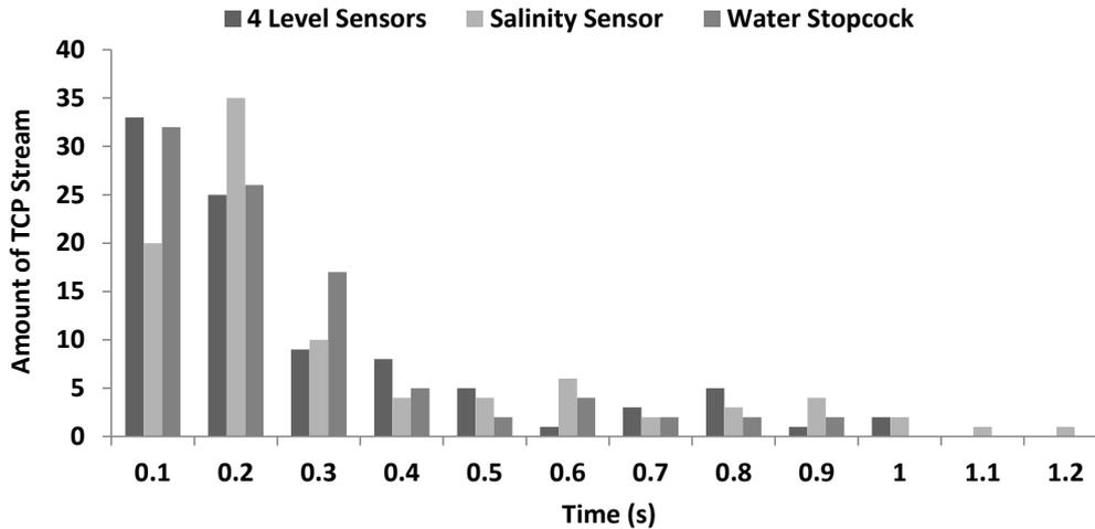
Fig. 18. Histogram of the delay between TCP messages.
