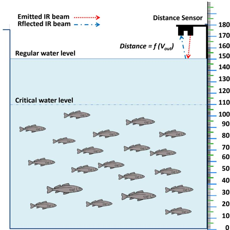
Fig. 5 Distance sensor position in fish tanks
