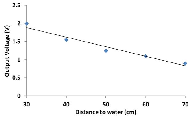
Fig. 6 Distance to water vs. output voltage.
