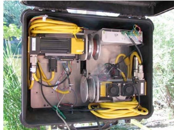
(b) Motor system actuating the mobile robot
