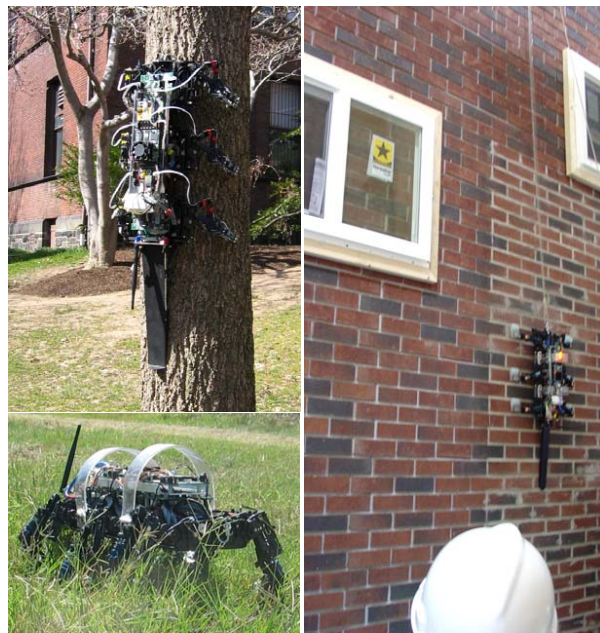
Figure 7: The RiSE platform is capable of scaling a wide variety of real world surface types and variations as well as maintaining capable level ground locomotion. Clockwise from the upper left, RiSE is climbing a tree, climbing a brick wall, and walking through tall grass.
