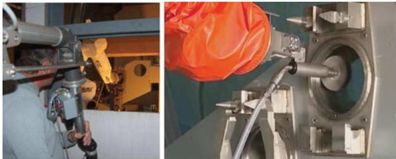
Figure 16. Brushing task on the mock-up.
