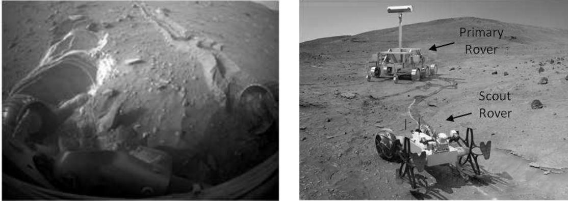
Figure 1: Image of MER Spirit stuck on soft soil (left), courtesy of NASA (NASA, 2010), and conceptual illustration of the FASTER mission scenario (right), courtesy of the FASTER consortium (FASTER, 2013)
