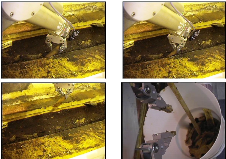
Figure 11: Romain 50 arm working on the cell threshold
