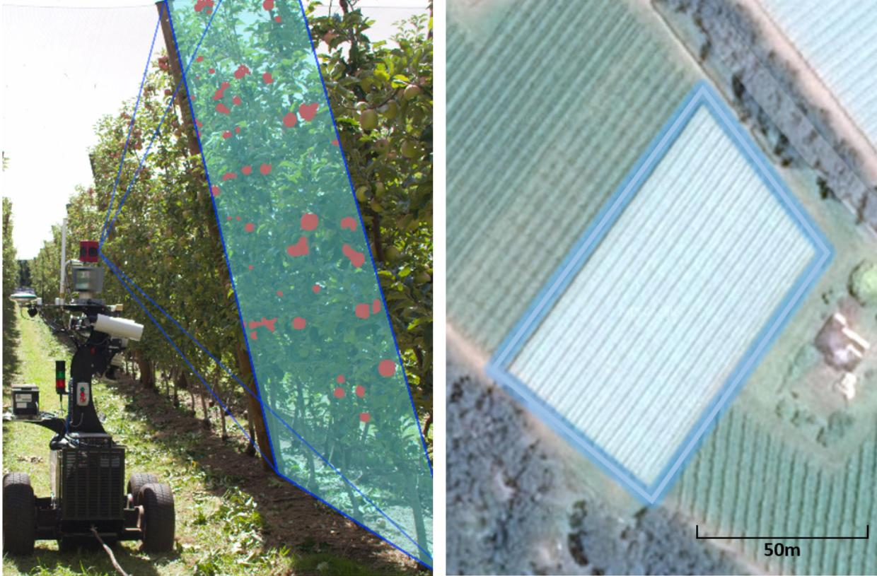
Figure 1: Left: The research ground vehicle Shrimp traversing between rows at an apple orchard, capturing tree image data. Location of apples manually illustrated in the field of view of the camera. Right: Satellite view of the 0.5 *ha* orchard test block.
