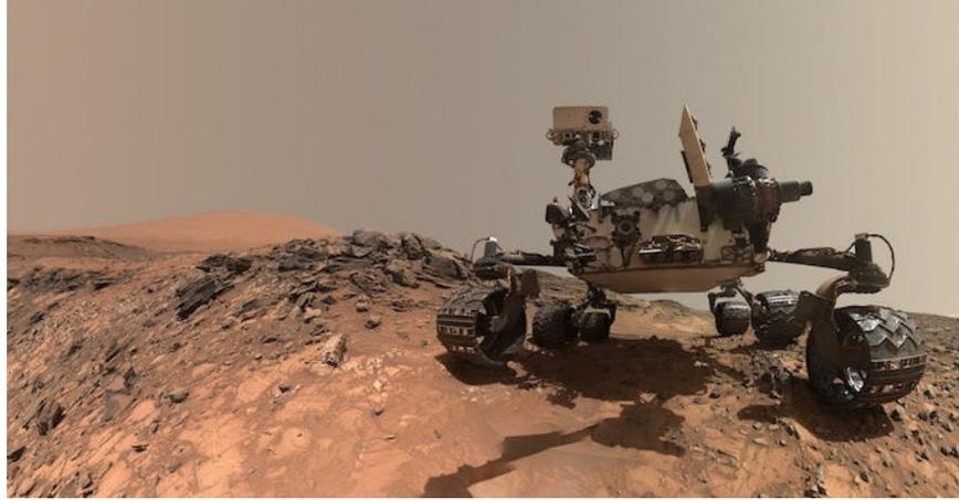
Figure 1: Self-portrait of the MSL Curiosity rover, taken on Sol 1065. Sufficient clearance between the vehicle and the ground is necessary to safely traverse on rough terrain with outcrops. (Credit: NASA/JPL-Caltech/MSSS)
