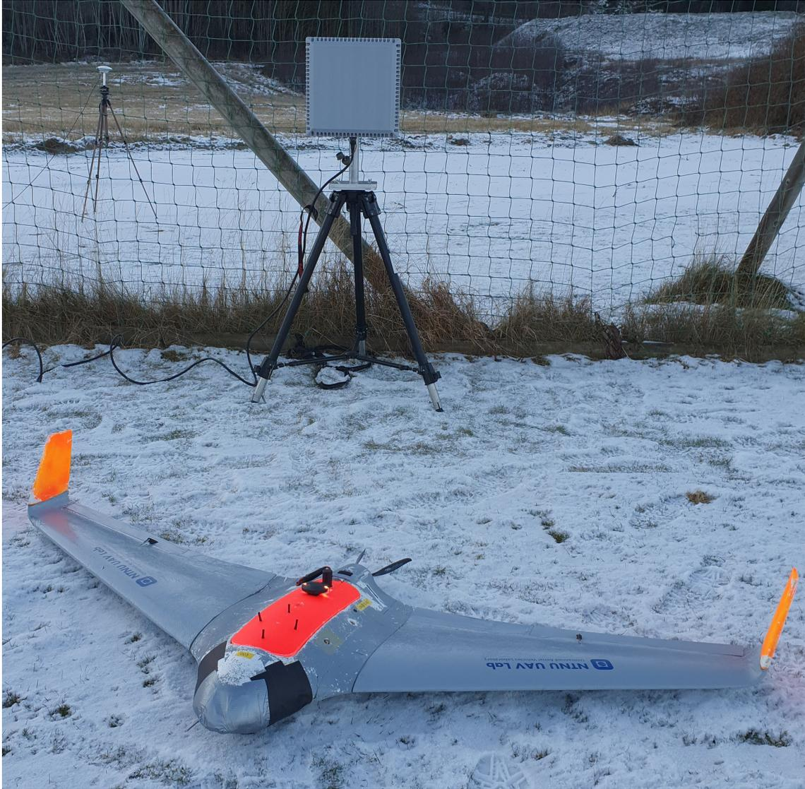
Figure 5: The four UAV antennas mounted in a diamond shape in the front part of the orange lid on the Skywalker X8, with the base antenna in the background
