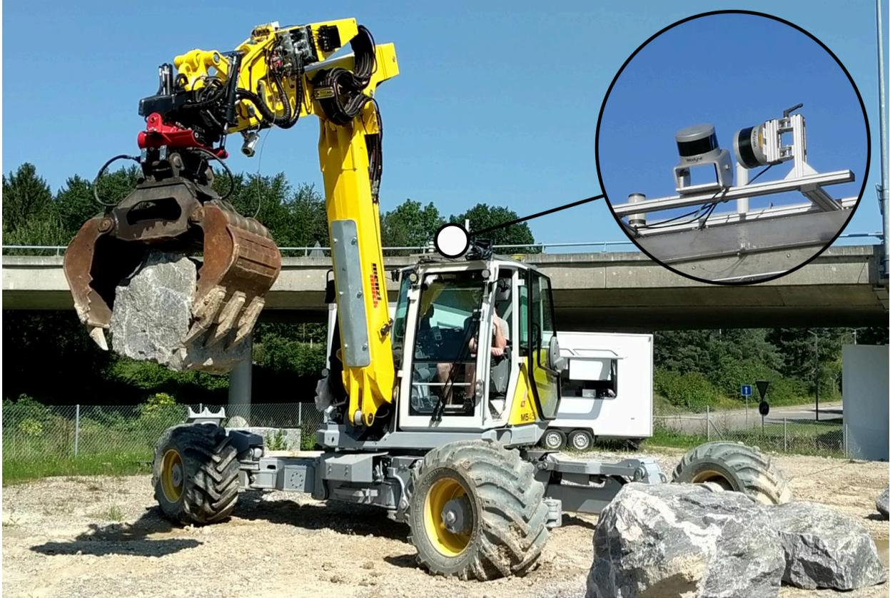
Figure 2: HEAP is an autonomous walking excavator based on a highly customized Menzi Muck M545. It is equipped with onboard sensors for state estimation (GNSS, IMUs, and encoders) and scanning the environment (3D LiDARs). As shown in the inset, the two LiDARs are mounted perpendicularly to each other such that a scanning motion is achieved not only while driving the robot around, but also while swinging the cabin.
