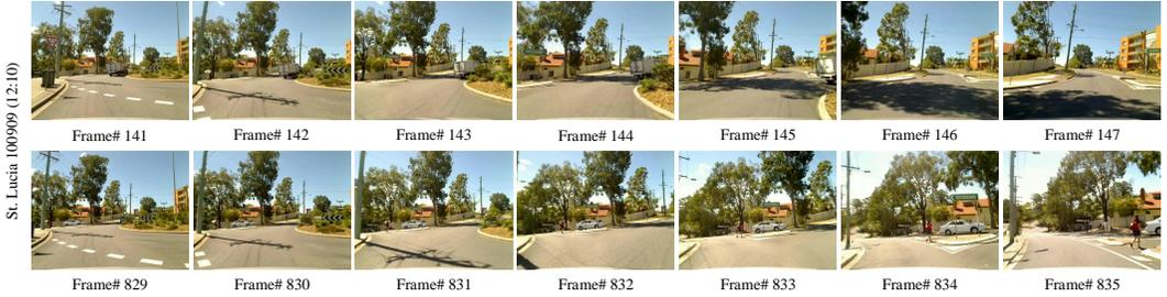
**FIGURE 4** A labeling correction: the image sequence in the first row shows the robot’s trajectory as it turns to the right road, while in the second row, it turns to the left road at the same place. Frames #835 and #147 are visually different but are labeled as loops according to the GPS, for its distance is lower than 10 *m*. During our experiments, these images are considered as true negative pairs.
