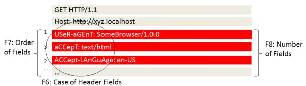
Fig. 14 Three steganographic methods applied to the HTTP request header
