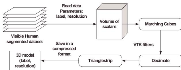
Fig. 2. Reconstruction of surface models
