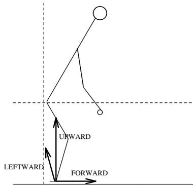
Figure 1: The Body Coordinate Frame
