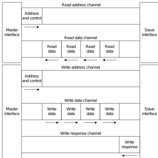
FIGURE 2 Channels in AXI interface, taken from [26].
