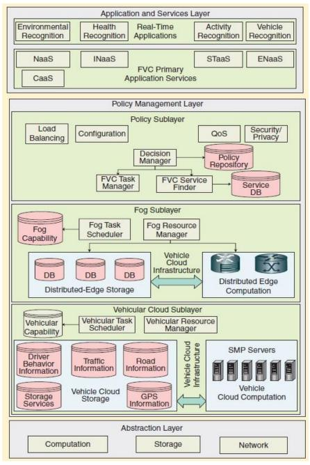
Figure 3: Fog Vehicular Computing Architecture
