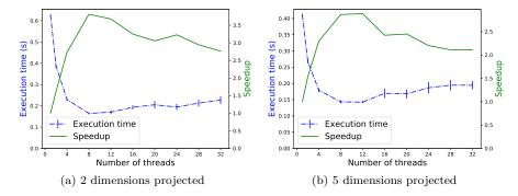
Figure 4: Computation time and speedup for 20 projections of polyhedra with 9 constraints with no redundant constraints and 16 variables, on Paranoia (20 hyperthreaded cores, OpenMP). Each parametric linear program has 2–36 regions
