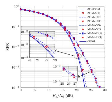
Fig. 3: SER of GFDM (with MF and ZF receivers) and of OFDM. Legend: S=simulation and T=theory.
