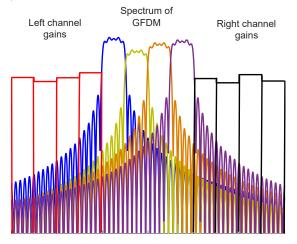
Fig. 2: PSD of GFDM and left and right channel gains for four subcarriers.
