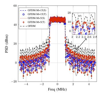
Fig. 4: PSDs of GFDM and OFDM signals.
