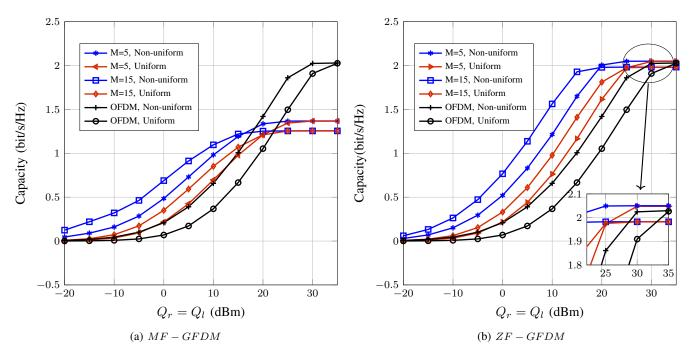
Fig. 6: Total sum rate of the SU of GFDM with MF and ZF receivers in compare with OFDM.
