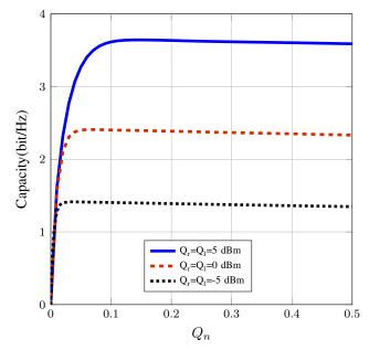
Fig. 5: Capacity of the GFDM with MF receiver versus  $Q_n$  for three constant interference power constraints.
