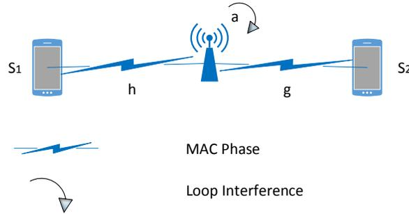
Fig. 1: A dual-hop non-orthogonal multiple access based full-duplex one-way wireless relaying network model.
