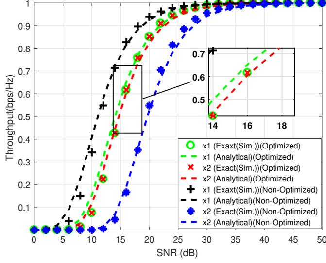
Fig. 10: The optimized and non-optimized throughput performance comparisons of  $x_1$  and  $x_2$ .
