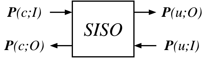
Fig. 3. The Soft-Input Soft-Output (SISO) module
