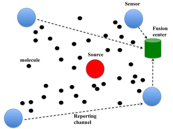
Fig. 1. System model: The molecular source that is to-be localized lies within the convex hull of the nano sensor/anchor nodes (each of which receives the molecules emitted by the source). Moreover, the sensor nodes report their measurements to a fusion center which ultimately does the signal processing to localize the source.
