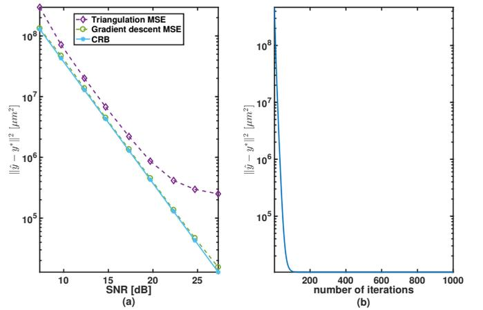
Fig. 3. (a) Gradient-descent method outperforms the triangulation method for whole range of interest of SNR values, (b) the squared error of the gradient-descent method decreases monotonically with number of iterations  $k$ .
