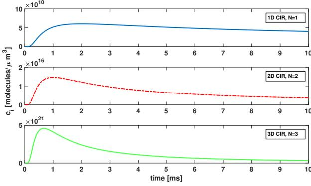
Fig. 2. The received molecular pulse/CIR at  $i$ -th sensor that is  $d_i = 2 \mu\text{m}$  away from the molecular source (for  $Q = 5 \times 10^5$ ,  $D = 1e - 9 \text{ m}^2/\text{sec}$ ).
