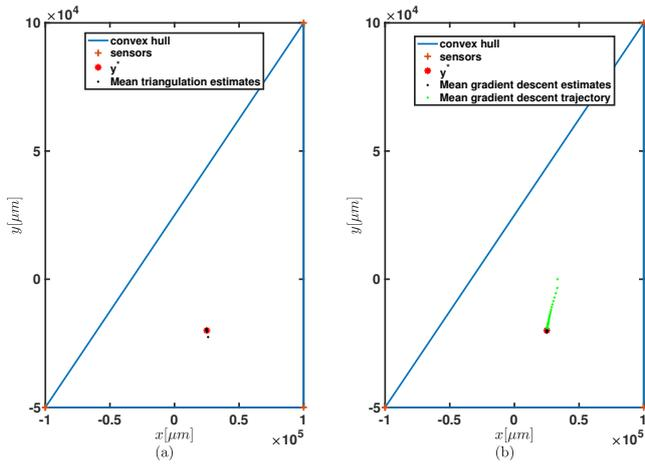
Fig. 4. Consider a 2D layout with the source lying within the convex hull of the  $n = 3$  sensors. (a) the location estimate provided by the triangulation method is quite close to the true source location, (b) the iterates of the location estimate provided by the gradient-descent method converge to the true source location uniformly.
