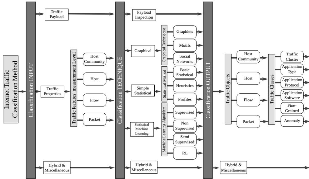
Figure 6. A multilevel taxonomy of traffic classification methods [48].
