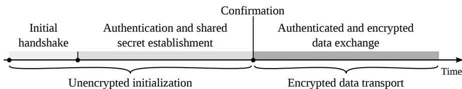
Figure 1. A general scheme of network security protocols.
