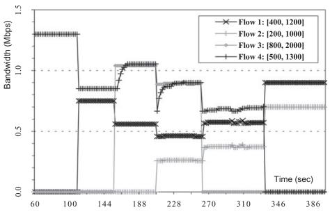
Figure 6. Example of resource distribution using the X-BDS approach
