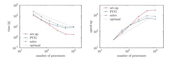
Figure 13. Strong scaling test for the problem of the *Bedřichov tunnel* containing 2D and 3D elements and 7.8M unknowns, computational time (left) and speed-up (right) separately for set-up and PCG phases, and their sum (solve).
