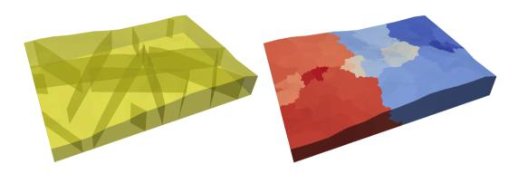
Figure 11. The *Bedřichov tunnel* problem; the system of fractures (left) and an example division into 256 substructures (right).
