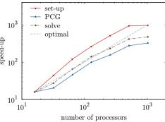
Figure 9. Strong scaling test for the problem of the *Melechov locality* containing 2D and 3D elements and 15M unknowns, computational time (left) and speed-up (right) separately for set-up and PCG phases, and their sum (solve).
