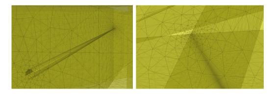
Figure 12. Example of difficulties in the mesh of the *Bedřichov tunnel* problem; detail of the tunnel geometry with fine elements (left) and enforced refinement at an intersection of fractures (right).
