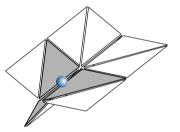
Figure 1. Example of a two-dimensional problem: even single fracture gives rise to two components of the two-dimensional mesh (left); example of three (shaded) triangles sharing a single Lagrange multiplier in 3D (right).
