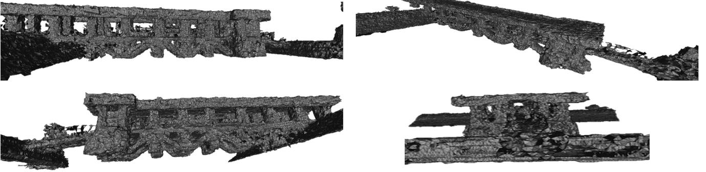
Figure 14: The mesh-based high quality map for the above-water part of the jetty, using a low probability threshold for occupied cells and the ball pivoting surface reconstruction algorithm. Cell-size=8cm.
