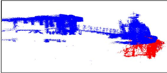
(c) Above- and below-water parts of marine structure, point cloud-based map. In red color below water part, in blue color above water part.
