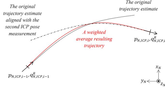
Figure 4: The principle of *trajectory approach*: when the new ICP measurement arrives (time-step  $i$ ), trajectory estimate based on measurements other than ICP (black dotted line) is duplicated and aligned with the incoming ICP measurement (black dashed line) and weighted average (red solid line) of these two trajectories is computed.
