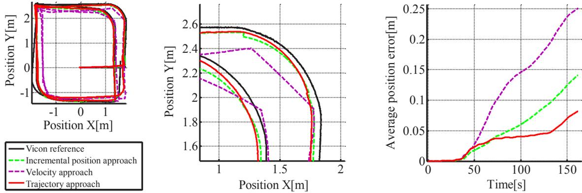
Figure 15: Comparison of effects of the three different ICP aiding approaches on the estimated trajectory (left, middle) and on the average position error (right). Note the *corner cutting* effect of the *velocity approach*.
