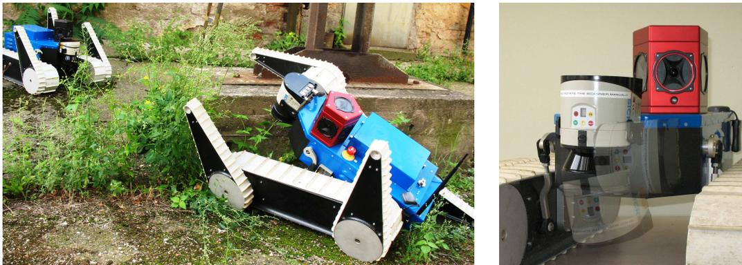
Figure 1: Picture of two USAR UGVs used for experimental evaluation (FP7-ICT-247870 NIFTi project) and a detail of the sensor setup (a PointGrey Ladybug 3 omnidirectional camera and a rotating SICK LMS-151 laser range finder). See Section 3.1 for more details.
