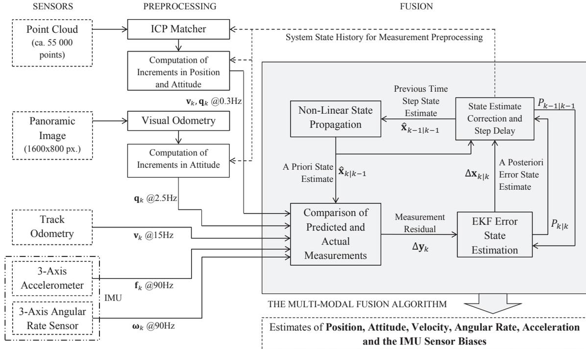
Figure 2: The scheme of the proposed multi-modal data fusion system ( $\boldsymbol{\omega}$  is angular velocity,  $\mathbf{f}$  is specific force (Savage, 1998),  $\mathbf{v}$  is velocity and  $\mathbf{q}$  is quaternion representing attitude).
