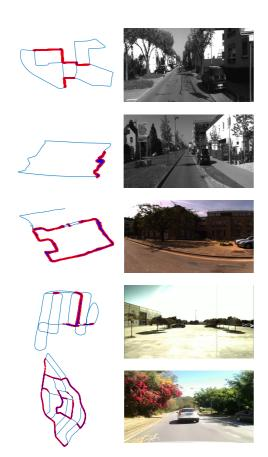
**FIGURE 12** Robot trajectories (left) and example images (right). From top to bottom: KITTI 00 (Geiger et al., 2012), KITTI 06 (Geiger et al., 2012), City Center (Cummins and Newman, 2008), Malaga6L (Blanco et al., 2009), St. Lucia 100909 (12:10) (Glover et al., 2010). The loop closure detections are labelled using red circles.
