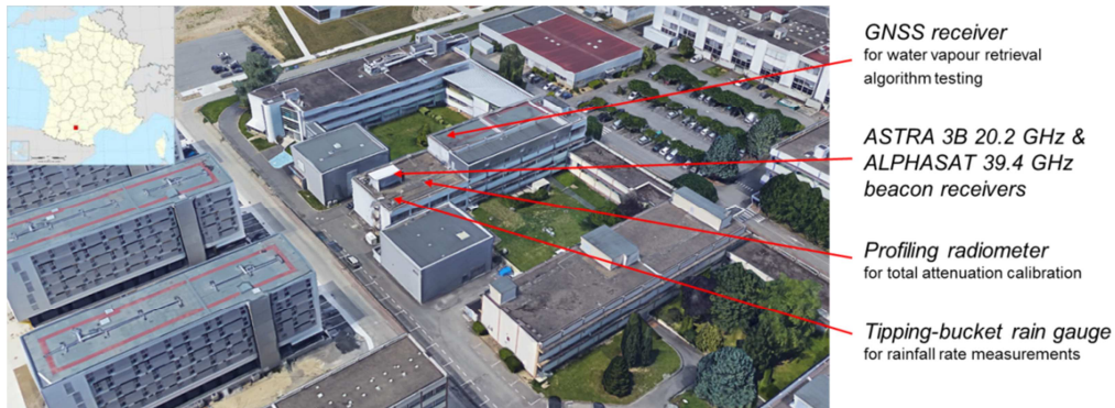
Figure 1. Overview of the Ka and Q band propagation experiments in Toulouse, France
