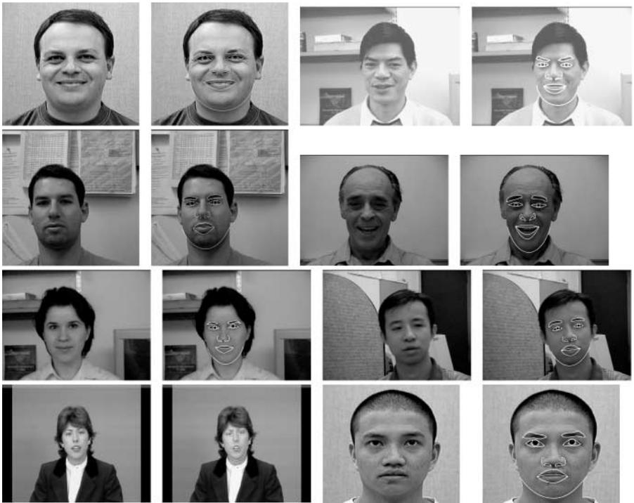
**FIG. 23.** From top left to bottom right: Mario, Guan, Dima, Stan, Dana, Xun, Claire, and Alau. In each box: original frame (left); feature shape detected (right).
