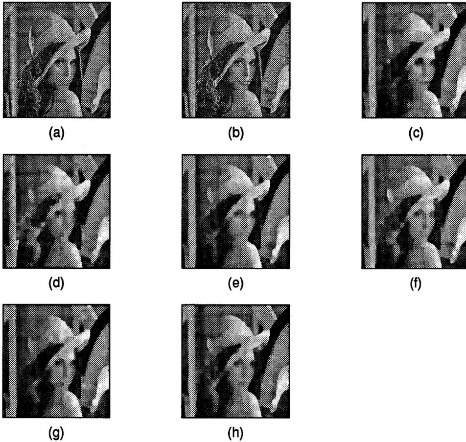
FIG. 2. (a) Grayscale “Lena” image, (b) a version corrupted by Gaussian noise ( $\sigma = 10$ ), and filtered results from (c) opening–closing by  $7 \times 7$  structuring element, (d) closing–opening by  $7 \times 7$  structuring element, (e) type-I, (f) type-II, (g) type-V, and (h) type-VI ASFs.
