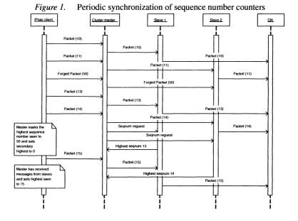
After the packet with sequence number 14, the master sends the periodic sequence number synchronization request to all slaves. When the master sends
