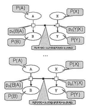
Figure 3. Different probability tables corresponding to different contexts are associated with vertexes of the second-level Bayesian network
