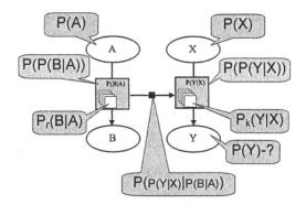
*Figure 1.* The sample of a Bayesian C-Metanetwork. The nodes of the 2nd-level network correspond to the conditional probabilities of the 1st-level network P(B|A) and P(Y|X). The directed arc in the 2nd-level network corresponds to the conditional probability P(P(Y|X)|P(B|A))
