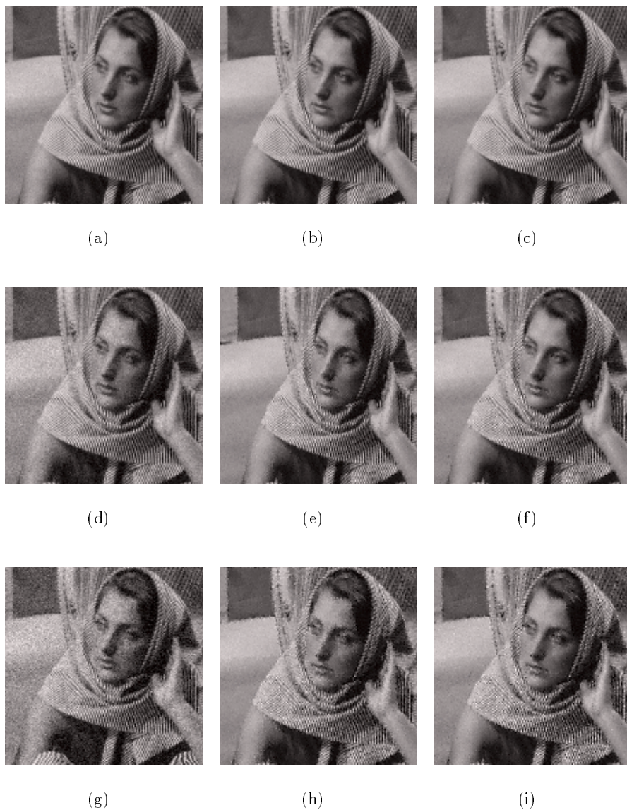
Fig.8. Test on visibility of embedding of Gaussian distributed watermark: direct embedding according to scheme (1) with the watermark strength 5 (a), 10 ( d) and 15 (g); and adaptive schemes with NVF (23) (b, e, h) and NVF (26) (c, f, i) with the corresponding watermark strengths given in Table (2).
