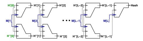
Fig. 3. The Double-Pipe Hash
