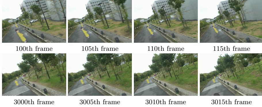
Fig. 6. Match move using estimated extrinsic parameters.
