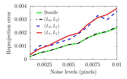
Figure 6: Reprojection errors for camera resectioning.
