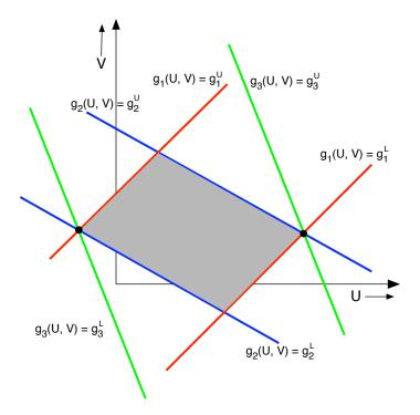
Figure 3: The red lines indicate the lower and upper bounds on the denominator  $g_1$  while the blue lines indicate bounds on the denominator  $g_2$ . The shaded gray region represents the induced bounds on the variables U and V. Any linear function of U and V restricted to the domain represented by the gray polygon will attain its extremal values at two vertices of this simplex, as illustrated by the thick black points for some linear function  $g_3(U, V)$  represented by the green lines.
