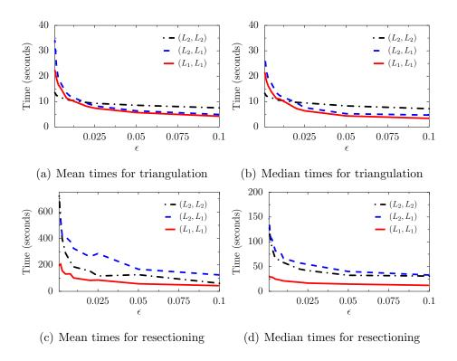
Figure 7: (a) and (b) show trends for the mean and median times, respectively, over 200 trials, for termination of the triangulation algorithm as the optimality tolerance,  $\epsilon$ , is varied from 0.01 to 0.1. (c) and (d) show the same for the resectioning experiment.
