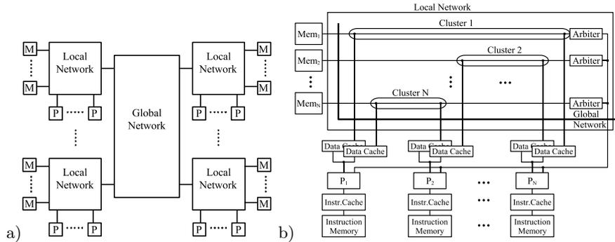
**Fig. 1.** General system structure (a) and architecture of a single SoC module (b)
