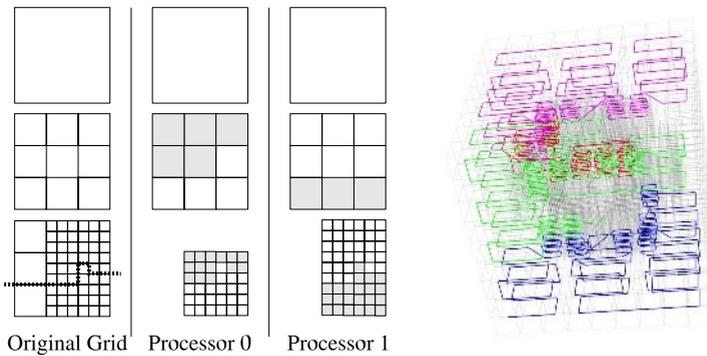
**Fig. 3.** The left-hand side shows a domain decomposition into two hierarchical partitions. The grey cells are held on a processor, but not evaluated since they do not belong to the processor (passive elements). The example on the right-hand side just gives an idea how a three-dimensional partitioning might look like.
