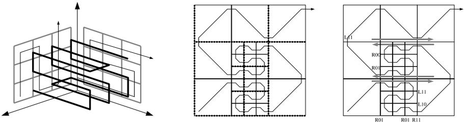
**Fig. 2.** On the left-hand side one can see the projection property, i.e. the projections of the Peano curve are again Peano curves. In the middle the alternating edge colouration is illustrated (even/odd indicated by dotted/solid), whereas on the right-hand side one can observe the palindrom / stack property (fat arrows). To some vertices their classifier value  $c$  is added.
