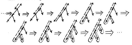
That is, we distinguish during traversal of the tree between a *leftdown* phase and a backup phase.
