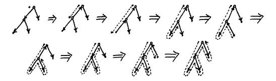
Since each arrow changes exactly twice of direction, the net result of the traversal is no change at all: at the end the original tree is recovered.
