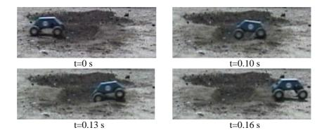
Fig. 12. Photo series of high-speed ditch traversal (7.4 m/s)
