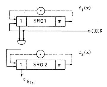
If we are only interested to generate the sequence  $b_{G(k)}$ , we use the generator of example 2. This structure works in the following manner: Generates shiftregister 1 an 1 the register SRG 2 is shifted and the output of SRG 2 is used for the output of the generator. Otherwise SRG 2 is not shifted and the previous generated bit of SRG 2 is used as output bit.
