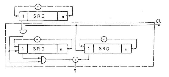
The sequences of example 1 have bad pseudo-noise properties, because the frequency of 1's at the output is only 1/4. To remove this defect we add (mod 2) another linear shiftregister sequence to the sequence  $(c_k)$ . If we assume (m,n) = 1 the following Lemma shows that the resulting sequence has better pseudo-noise properties.
