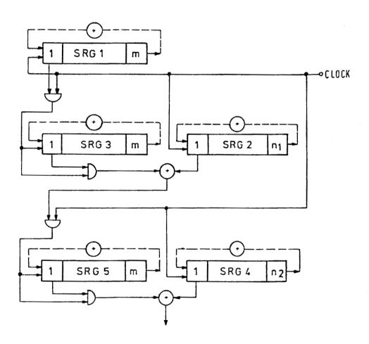
This example shows how a repetition of the method of example 1 leads to sequences of very high complexity. If we assume that all feedback polynoms are primitive polynoms, it is possible to proof that in each stage the number of 1's is relatively prime to  $2^m$  -I. The output sequence of this structure has the least period  $(2^m - 1)^3$ .  $(2^{n_1} - 1) \cdot (2^{n_2} - 1)$  if all the starting vektors of all registers are not equal 0.
