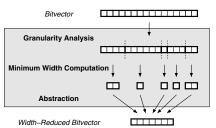
of a variable into a sequence of chunks is called a granularity. For each such chunk of a signal, the necessary minimum width is computed, as required by dynamical data dependencies. According to these computed minimum chunk widths, the reduced width for the corresponding shrunken signal is reassembled (see [7,8] for further details on the reduction).
