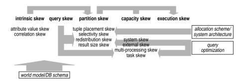
Fig. 3. Overview of skew causes
