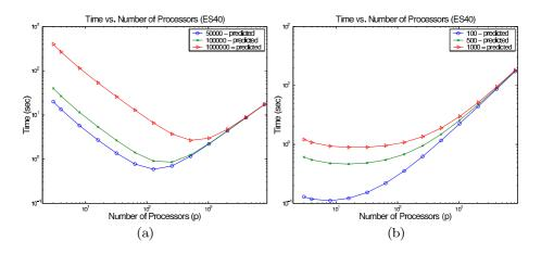
Fig. 4. Expected cycle times on larger ES40 systems for strong (a) and weak (b) scaling
