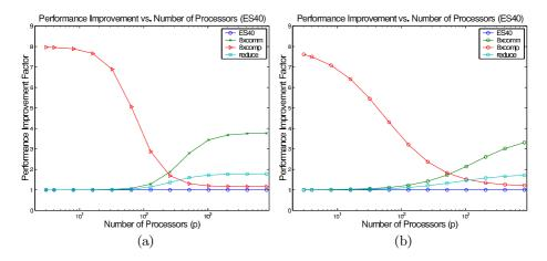
Fig. 5. Relative impact of improved computation and communication capabilities for strong (a) and weak (b) scaling
