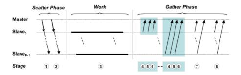
Fig. 2. Communication pattern for a single cycle of MCNP
