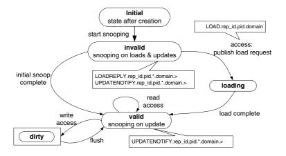
Fig. 6. Snooping states of the data container
