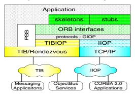
Fig. 2. ObjectBus Architecture
