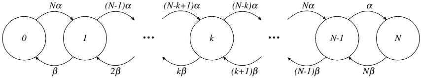
**Fig. 2.** Aggregated state-transition diagram of the GMPLS queueing model.
