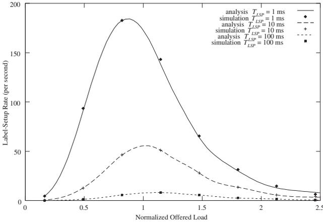
**Fig. 4.** Label-setup rate as a function of normalized offered load with  $T_{rel} = 1$  ms and  $m = 3$  under different  $T_{LSP}$ .
