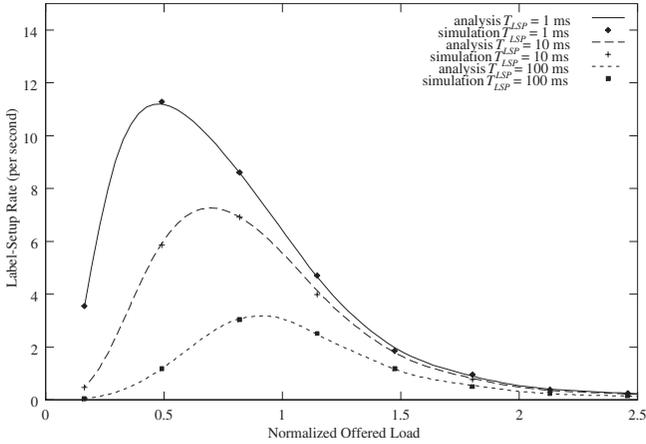
**Fig. 5.** Label-setup rate as a function of normalized offered load with  $T_{rel} = 50$  ms and  $m = 3$  under different  $T_{LSP}$ .
