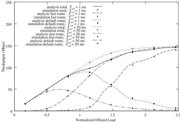
**Fig. 7.** Throughput as a function of normalized offered load with  $T_{LSP} = 100$  ms and  $m = 3$  under different  $T_{rel}$ .
