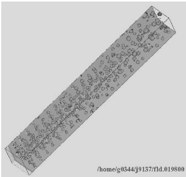
Fig. 6. Example of monitoring using AVS/Express (two-phase flow in a pipe)
